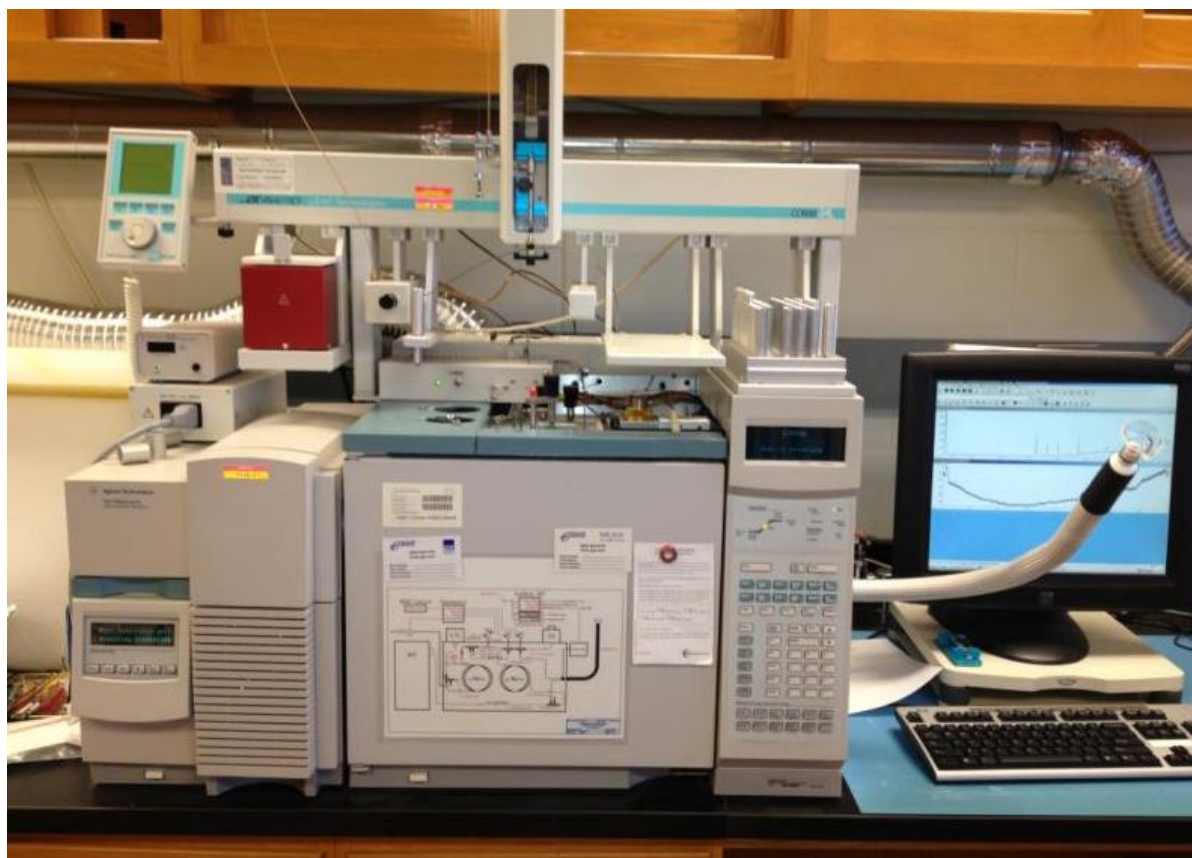
Figure 5. Multi-dimensional gas chromatography-olfactometry system at Iowa State University.
