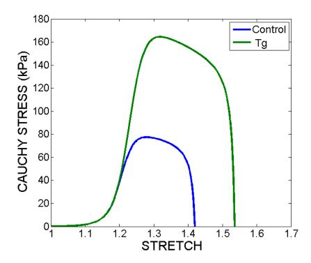
Figure 7-12. Theoretical change in the uniaxial tensile response between the control and Tg-crosslinked TEBVs.
