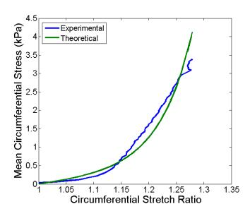
Figure 6-15. Verification of the proposed strain energy function. Comparson of the experimental and theoretical stress-stretch response of a tubular collagen gel.
