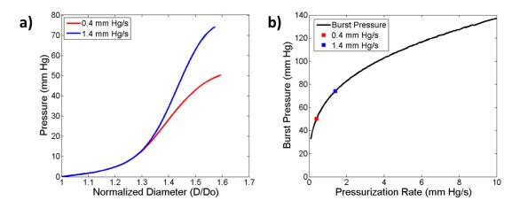
Figure 6-16. Predicted burst pressure test response.a) Pressure-normalized diameter and b) prediction of burst pressure with increasing inflation rate.
