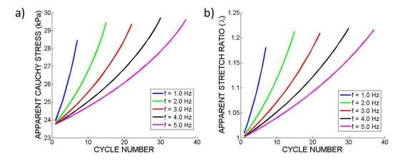
Figure 4-13. Effect of frequency on the apparent a) stress and b) stretch ratio with increasing cycle number.
