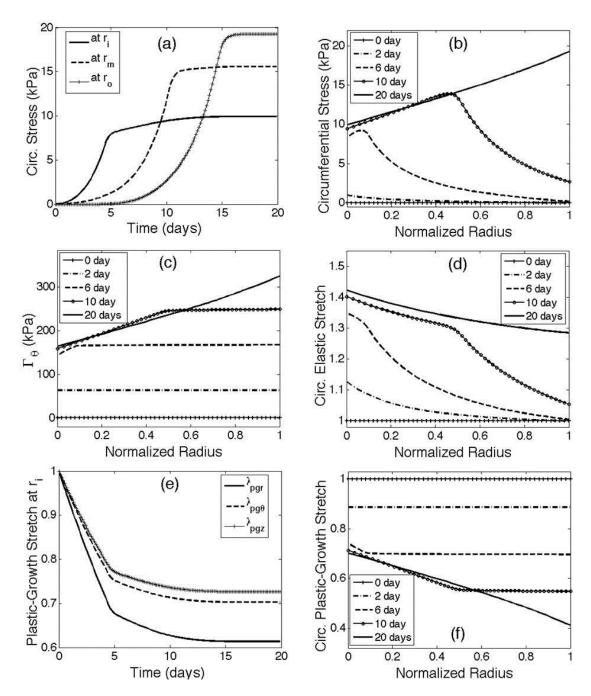
Figure 3-5. Evolution of mechanical properties over time in culture. Evolution of the local circumferential stress (a,b), circumferential damage and remodeling parameter  $\Gamma_{\theta}$  (c), distribution of the elastic stretch (d), plastic-growth stretches in the radial, circumferential, and axial directions (e), and distribution of the circumferential plastic-growth stretch versus radius at different time-points (f) for static culture on a mandrel.
