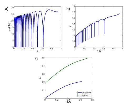
Figure 4-9. Modeling simulations of uniaxial cyclic loading.a) Stress-stretch response. b) Change in apparent stretch ratio and c) the loaded and unloaded stretch during the accumulation of damage.
