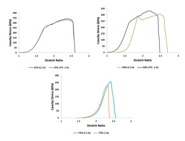
Figure 5-12. Effect of frequency during cyclic loading.
