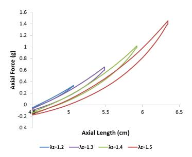
Figure 6-9. Axial force-length response at constant pressure.
