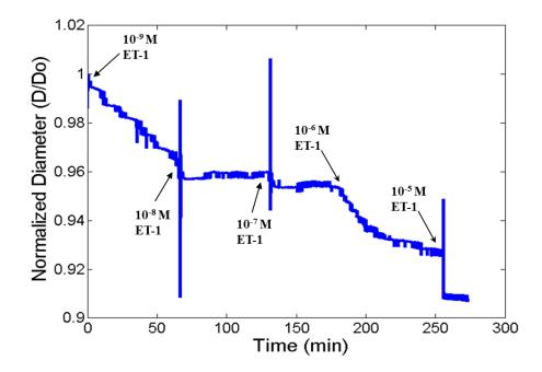
Figure 6-10. Functional testing of a collagen-based TEBV.Endothelin-1 (ET-1) was used as the vasoactive agent.
