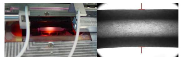
Figure 6-2. Image of a collagen gel TEBV undergoing biaxial mechanical testing. (a) Image of the vessel on the testing device. (b) Image of diameter measurement during mechanical testing.
