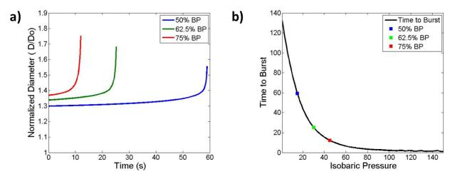
Figure 6-17. Predicted isobaric response of collagen gel TEBVs a) at 25 mm Hg, 30 mm Hg, and 35 mm Hg and b) predicted time to failure versus imposed pressure.
