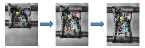
Figure 5-3. Manual tracking of the vessel during uniaxial testing.
