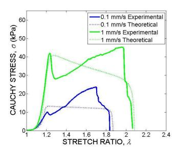
Figure 5-13. Experimentally and theoretically predicted stress-strain response during monotonic loading.
