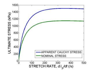
Figure 4-6. Predicted UTS with increasing stretching rates.
