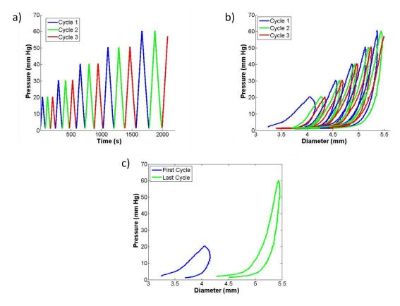
Figure 6-6. Biomechanical tests on collagen-based TEBVs. a) Testing protocol for the vessels. At a fixed length of  $\lambda_z = 1.10$ , the vessels were cyclically inflated at deflated to the pressures shown. b) Pressure-diameter response for the TEBVs. Note that the same color is used for the respective cycle for each pressure range. c) Change in diameter between the first and last complete cycle.
