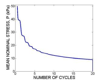
Figure 4-11. Nominal stress with increasing cycle number.
