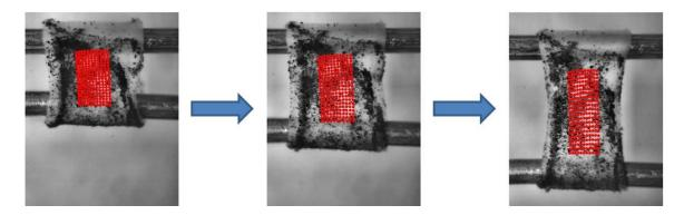
Figure 5-2. Tracking of the vessel using DIC during uniaxial testing.
