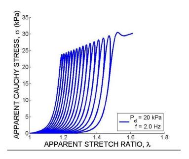
Figure 4-10. Apparent stress-stretch response during cyclic loading.
