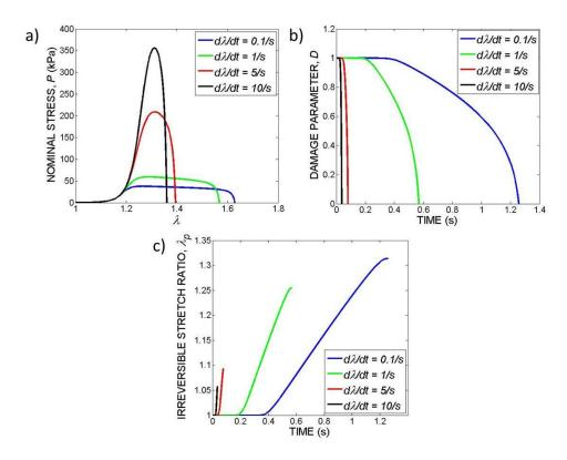
Figure 4-4. Modeling simulations of uniaxial tensile tests at different stretch rates.
