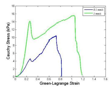
Figure 5-4. Representative Cauchy stress-Green strain curves for monotonic uniaxial tests performed at stretch rates of 1 mm/s and 1 mm/s
