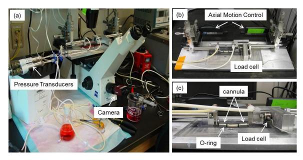
Figure 6-1. Biomechanical Testing System. (a) Computer controlled testing system capable of precise control of flow, pressure, and axial motion while monitoring diameter
