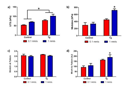
Figure 7-7. Uniaxial monotonic tensile tests performed on control and Tg-crosslinked TEBVs. a) UTS, b) modulus, c) stretch at failure, and d) work to failure are shown. Results are reported as mean  $\pm$  SEM (\*p<0.05).
