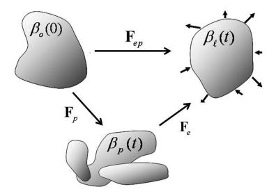
Figure 6-3. General kinematics for plastic deformation.
