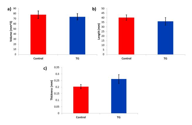
Figure 7-11. Changes in the geometric properties of control and Tg-treated collagen gel-based TEBVs. a) Volume, b) length, and c) thickness of control and Tg-treated vessels. Results are reported as mean  $\pm$  SEM. No significant differences were seen in any dimension.
