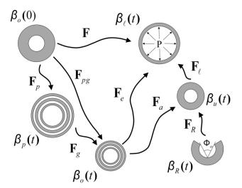
Figure 3-2. Kinematics of growth and plasticity of a thick-walled axisymmetric tube. Note that the configurations  $\beta_p(t)$  and  $\beta_o(t)$  consist of infinitesimally thin rings (each with thickness  $dR_p(t)$ ) that pass through radial location R(0) in  $\beta_o(0)$ ; since each ring is infinitesimally thin and cannot support a residual stress.
