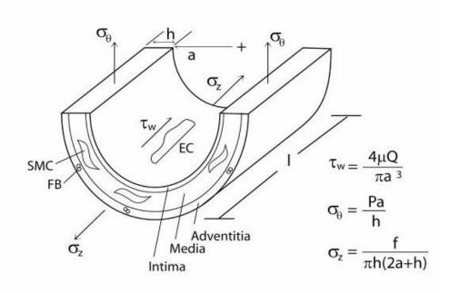
Figure 1-3. Forces on the the vascular wall. The blood vessel is exposed to three stresses: circumferential, axial, and shear. Taken from [53].
