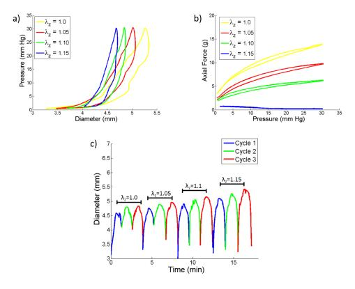
Figure 6-8. Effect of axial extension on pressure and axial load.a) Pressure-diameter and b) axial force-pressure responses of collagen-based TEBVs. Three pressure cycles of 0-30 were performed at  $\lambda_z = 1.00$ ,  $\lambda_z = 1.05$ ,  $\lambda_z = 1.10$ , abd  $\lambda_z = 1.15$ . Only the last cycle at each extension is shown. c) Change in diameter over each cycle. Note that the diameter at the maximum pressure of the last cycle increases with each extension.
