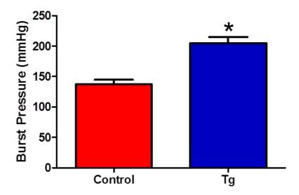
Figure 7-9. Burst pressure tests of control and Tg-treated collagen gel TEBVs. Results are reported as mean  $\pm$  SEM (\*p<0.05).
