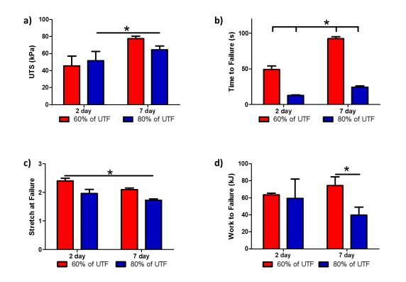
Figure 7-2. Uniaxial creep tests performed at 2 and 7 days of static culture. a) UTS, b) time to failure, c) stretch at failure, and d) work to failure are shown. Results are reported as mean  $\pm$  SEM (\*p<0.05).
