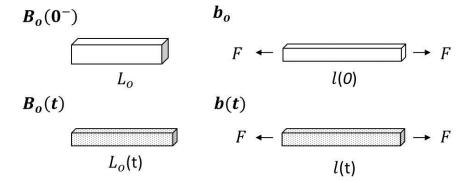
Figure 4-1. Uniaxial Kinematics. Schematic of the initial unloaded state  $B_o(0)$ , the deformed state  $b_o$  due to the instantaneous elastic deformation, the deformed state b(t) that results from the accumulation of damage, and the unloaded state  $B_o(t)$  after the load in b(t) is removed.
