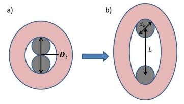
Figure 5-10. Estimation of stretch ratio using hook displacement.
