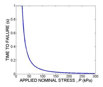
Figure 4-8. Predicted time to failure with increasing applied nominal stress.
