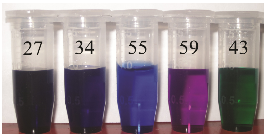
Figure 1. Candidate dyes and perceived luminance. Dyes in solution at equal concentrations (m/v) and physiological pH. From left to right: Evans Blue (chosen for use in our experiments), Coomassie blue, methylene blue, bromophenol blue, lissamine green. Perceived luminance values are provided above each dye. Lower luminance correlates with darker appearance.
