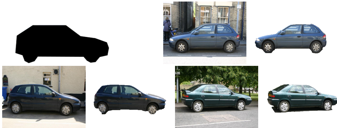
Figure 5.9: Template shape matching examples: shape (top left) and pairs of original images + segmentations with E_2(S) .
