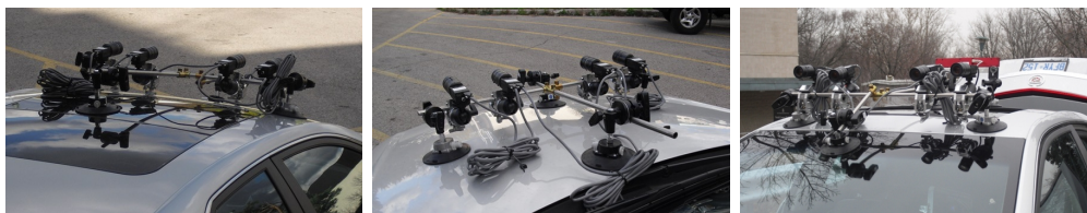
Figure 2.5: Various mounting configurations: a) (left): dual stereo sensors mounted on top of vehicle b) (center): dual stereo sensors mounted on hood of vehicle, c) (right): experiment with an external sensor configuration
