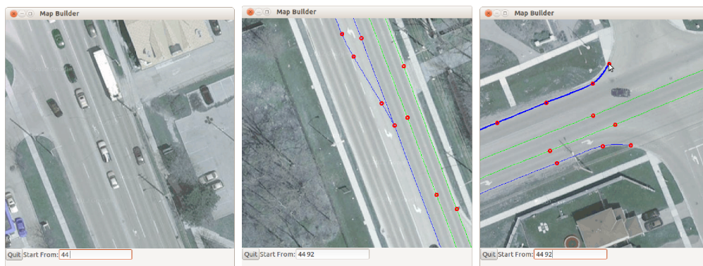
Figure 3.3: Images from the map building application a) (left): visible lanes in presence of traffic b) (center): Splitting lane sample c) (right): Several neighboring lanes
