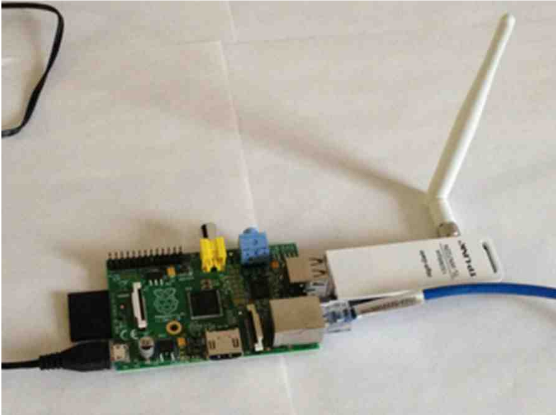
Figure 5-1: Prototype of Wi-Fi sensor
