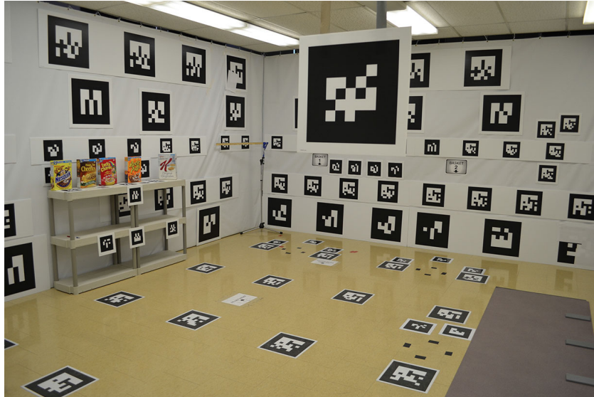
Figure 4.3: Physical space in which fiducial markers were setup in order to create a predefined multi-marker system.
