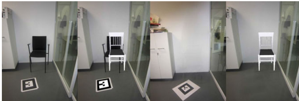
Figure 2.8: Diminished reality example, images from left to right: original, augmentation over existing object, diminished image, augmentation over diminished image. [25]
