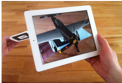
Figure 2.4: Apple iPad TM device augmenting a fiducial marker with a virtual object.
