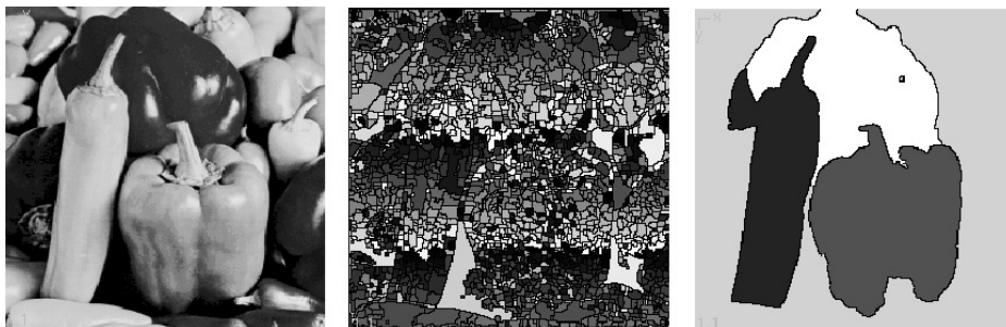
Figure 4.8: Left: original image, middle: row watershed segmentation, right: watershed segmentation using region marks to control over segmentation 4
