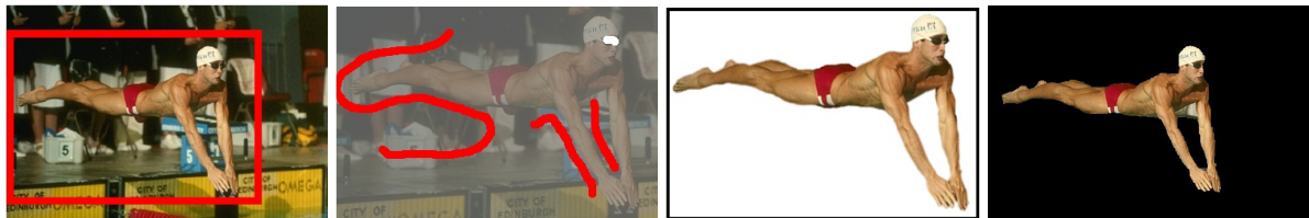
Figure 1.5: From left to right: grabcut initialization rectangle, grabcut user editing, grabcut segmentation result and our result
