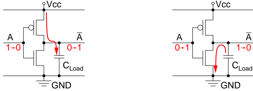
Figure 2.1: Output transitions of a CMOS inverter
