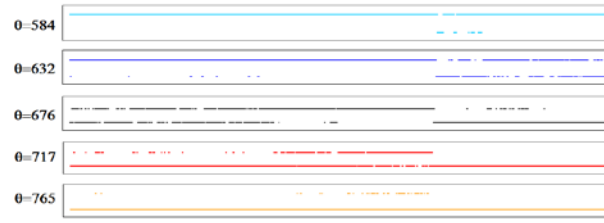
Figure 29. The signal x^{RR} symbolized via five different fixed partitions with thresholds set at \theta=584, 632, 676, 717, 765 . The corresponding colors of the plots are: turquoise, blue, black, red and orange
