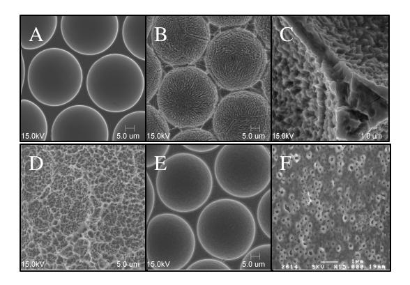
Figure 3-1 Surface nanoscale structures of titanium disks prepared using acid etching and electrochemical machining.
