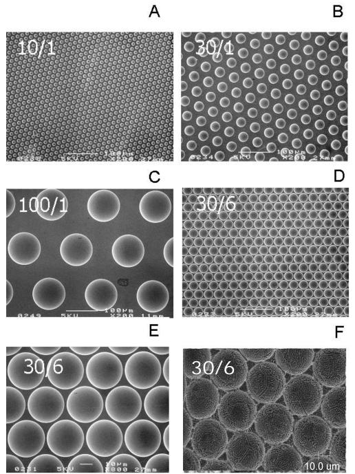
Figure 2-1 Surface microtopography of titanium disks.
