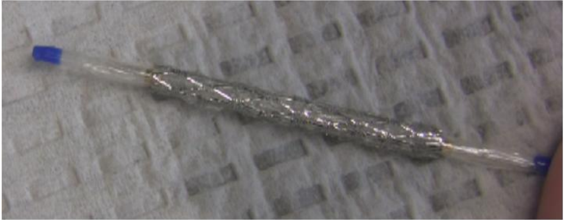
Figure 4.2: Crimped PVA cryogel covered stent on balloon catheter prior to expansion.
