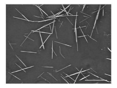
Figure 3.1. Micrograph of lipid microtubes formed from  $DC_{8,9}PC$  lipid in bright field microscopy, scale bar is 50 µm. Figure from Meilander et al., 2001.
