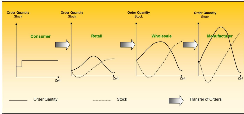
Figure 1.1: The bullwhip effect on demand at various stages of a distribution channel (Wikipedia). Zeit is German for time.
