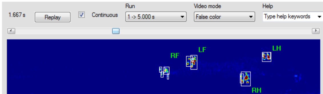
Figure B.1. Example of CatWalk analysis software screen. The video of a rat crossing the walkway is captured by the CatWalk system and can be displayed using the software. Limbs are labeled manually within the software, and then the intensity measurements are converted into quantitative data sets related to gait.
