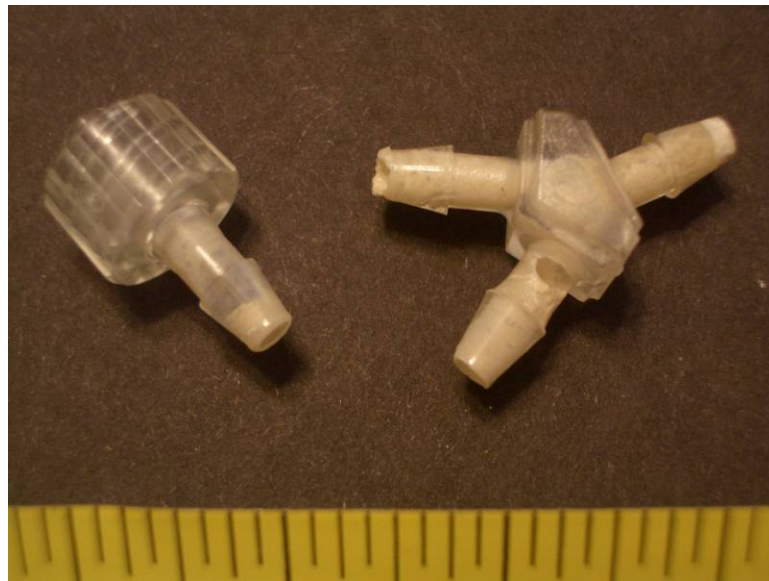
Figure 4.12: Disintegration of Connector and Coupling Walls. Walls of connectors and couplings disintegrated over time, possibly due to residual bleach or repeated autoclaving. Regular inspection and periodic replacement were necessary to avoid contamination due to connector and coupling disintegration. Ruler divisions are 1.6 mm.
