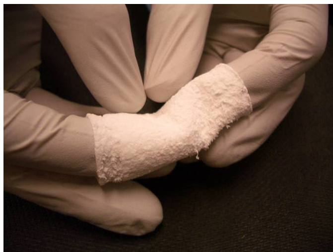
Figure 5.2: Large-diameter Porous Tubular Scaffold Composed of Poly(glycerol sebacate). Scaffolds with an inner diameter of 20 mm and wall thickness of 1 mm have been fabricated at lengths up to 75 cm.
