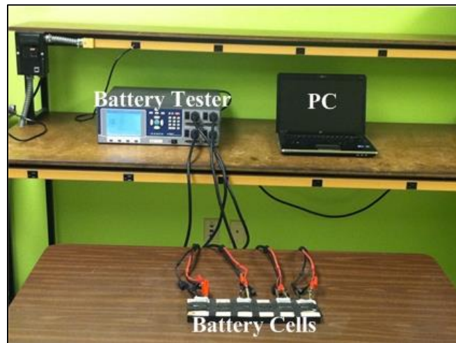
Figure 5.3: The experimental setup for electrical parameter and SOC estimation.
