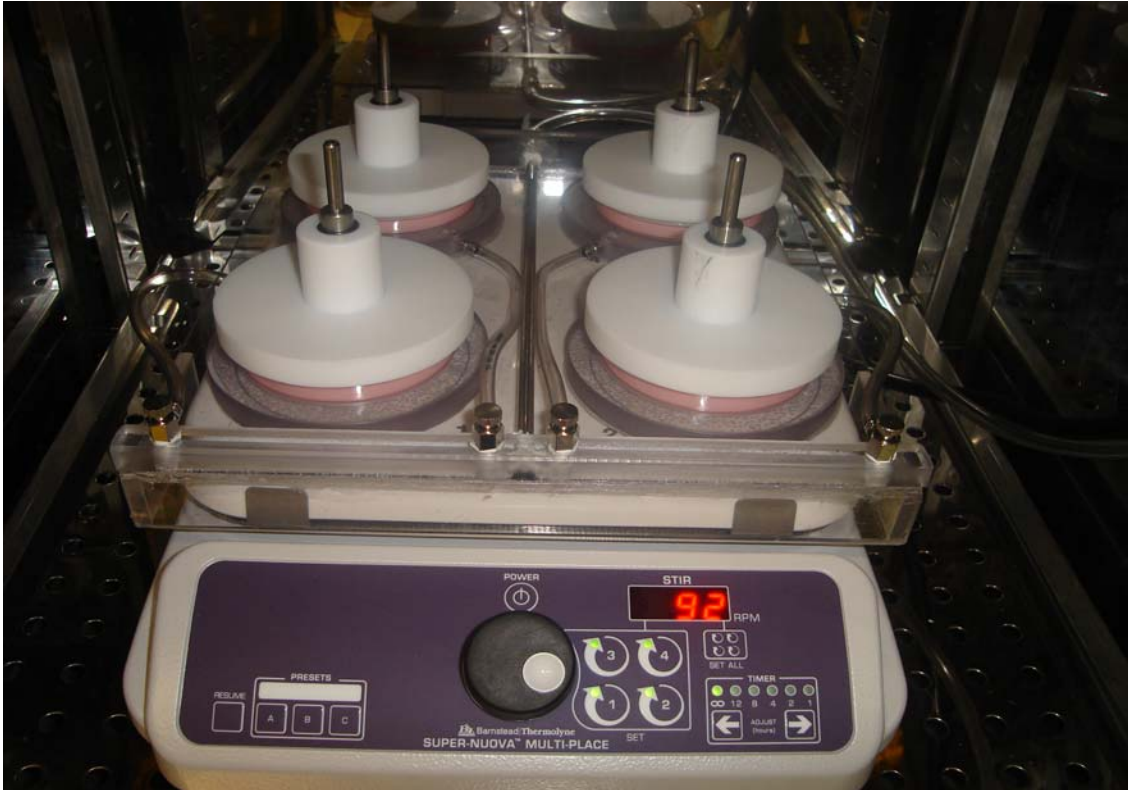
Figure 2.3. Photograph of Cone-Plate Shear Apparatus. This particular model can hold 4 separate cone-plate devices driven by a magnetic stir plate (cone contains a magnetic stir bar). Petrie dishes are securely suctioned onto a base plate via a vacuum pump to limit movement and curvature of the base of the Petrie dishes. For this study, two similar devices as shown above were available allowing for 8 concurrently sheared samples in a single experiment. Static control samples were cultured in the same incubator during shear.
