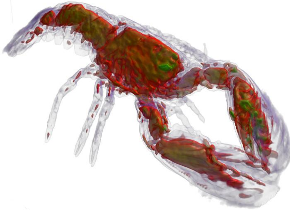
Figure 2-8 Example of volume rendering using ray casting. 8 bit CT volume of a lobster with dimensions of 301 x 324 x 56.
