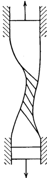
Figure 71: Lattice rotation due to fixed constraint at the specimen's shoulders [78]
