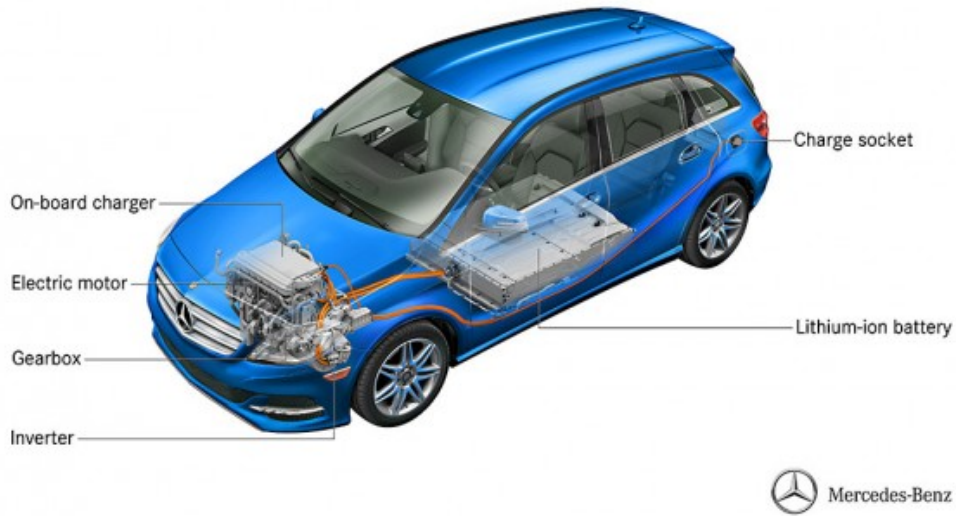
Figure 2.1: Power train diagram displaying the different components in the Mercedes 250e electric B-Class [26].
