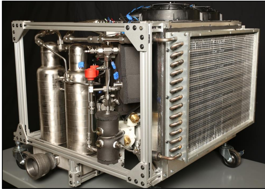
Figure 8.17: 2.63 kW cooling capacity chiller for diesel engine waste heat applications at severe ambient conditions (Ponkala et al. , 2018)
