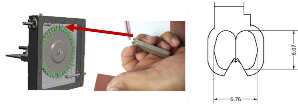
Figure 6.2: left: 3D printed Pelton turbine bucket, right: bucket dimensions in millimeters
