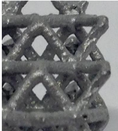
(a) Fabricated struts using SLM
