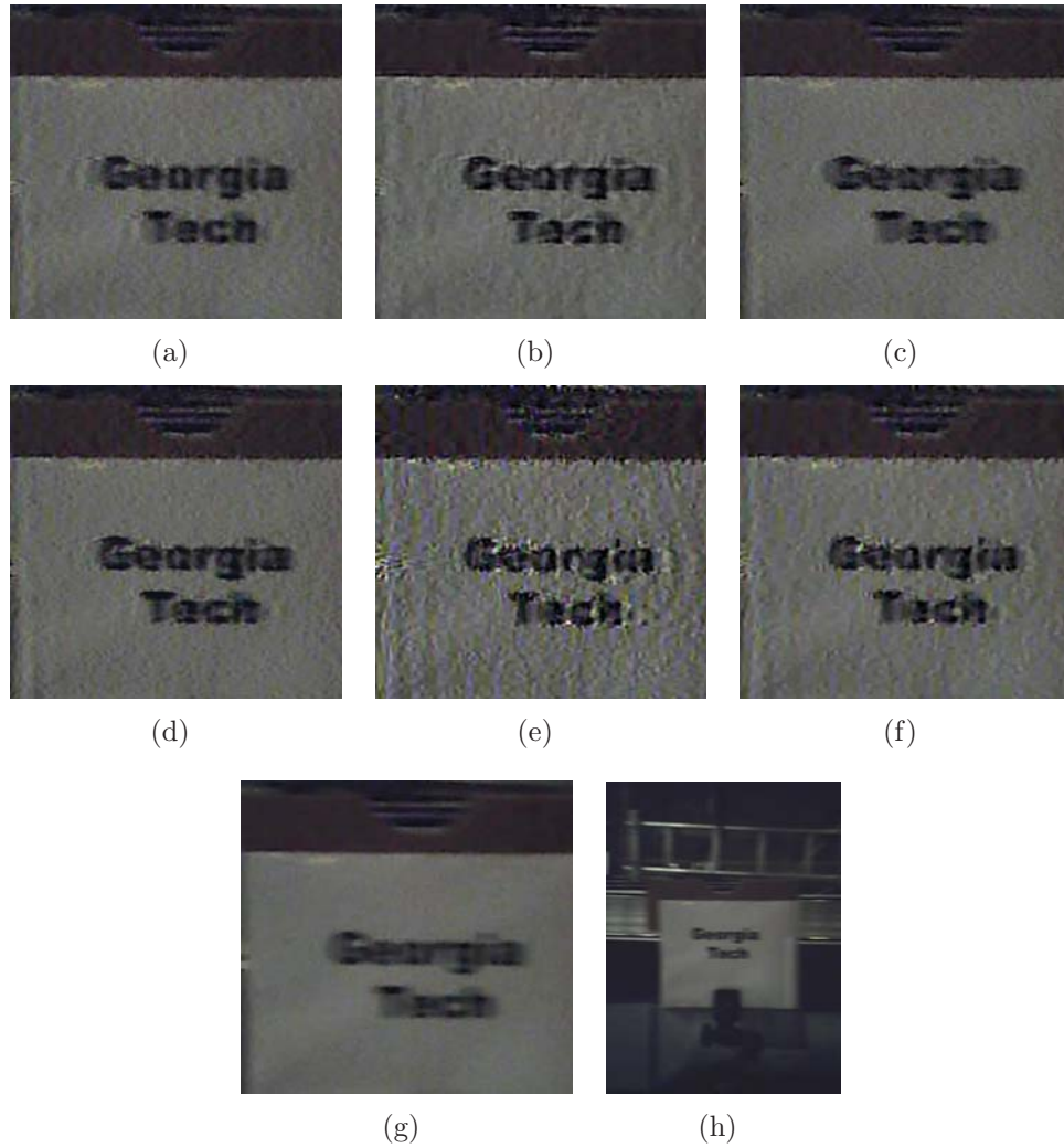
Figure 21: Test set #4. The obtained blurry image and estimated latent images by various methods. Images are taken at 10.4fps with periodic oscillatory input. Two PZT steps were used to create oscillatory response. (a) - (g) are cropped local images. (a) Proposed Method (b) Goldstein et al. (c) Fergus et al. (d) Whyte et al. (e) Shan et al. (f) Xu et al. (g) Cropped obtained blurry image (h) Obtained blurry image
