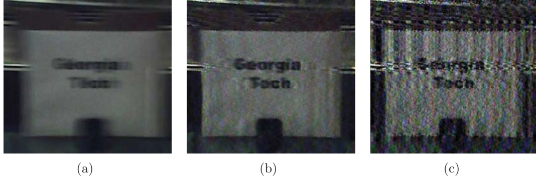
Figure 49: Comparison between Richardson-Lucy and Wiener deconvolution methods. The image was taken under low light condition to introduce noise and to test robustness. The results shows that the Richardson-Lucy method is robust to noise while the Wiener method is not. (a) Original blurry input (b) Result obtained by the Richardson-Lucy method (c) Result obtained by the Wiener method
