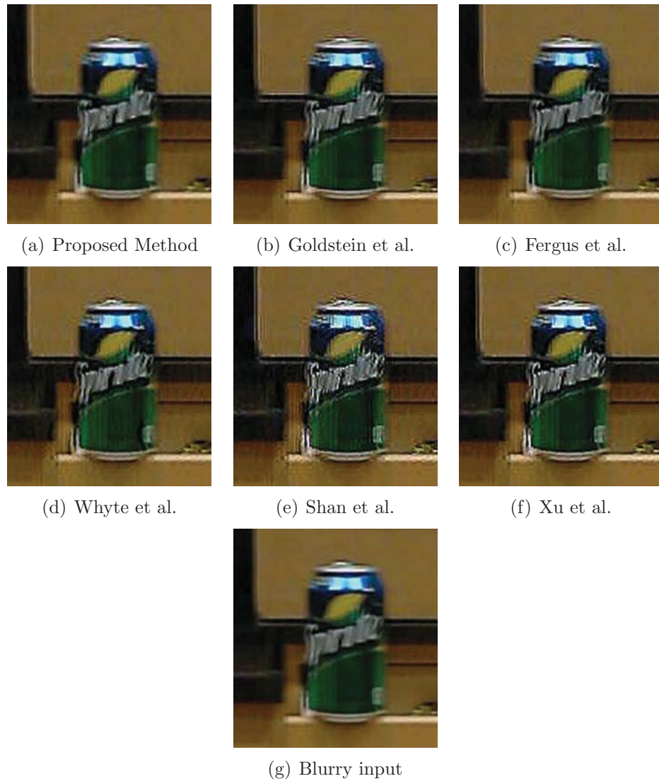
Figure 34: Test set #10. The obtained blurry image and estimated latent images by various methods. Images are taken at 29fps with Vibration Suppression input command. (a) - (g) are cropped local images.
