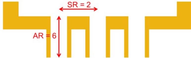
Figure 27. Schematic showing the preferred nozzle array design having a nozzle aspect-ratio of 6 and a nozzle spacing-to-diameter ratio of 2
