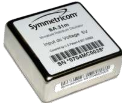
Figure 5: Symmetricom SA33.m rubidium clock
