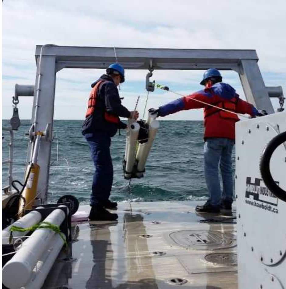
Figure 17: Float design, Revision 3 surfaced. The flotation members are connected at the bottom with two parallel plates, which mount the rod holding ballast weights below.
