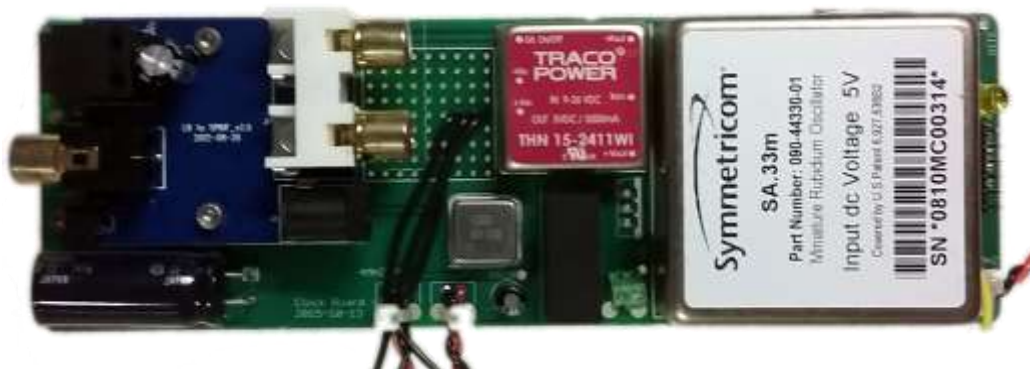
Figure 6: Clock circuit board. From left to right: S/PDIF converter, 4 MHz NAS clock, DC/DC converters, rubidium clock.
