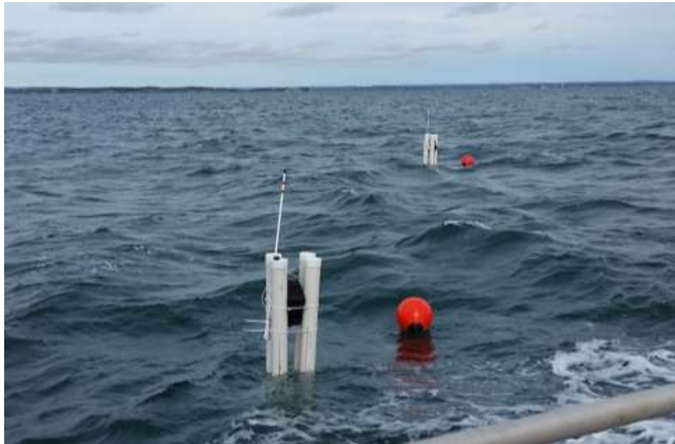
Figure 16: Float design, Revision 3. GPS antenna and waterproof box are mounted between flotation members.
