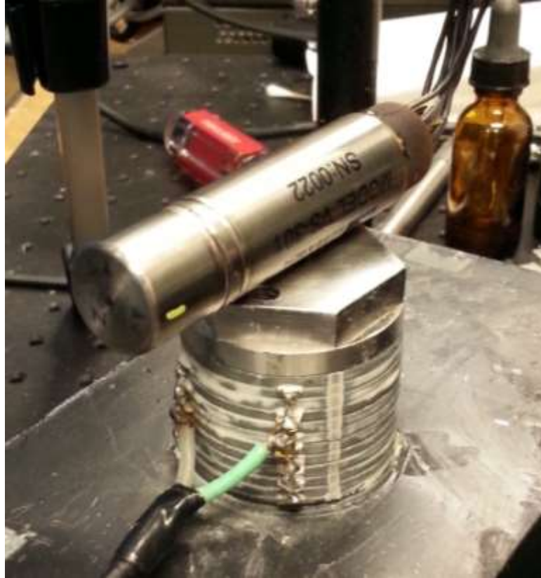
Figure 128: Radial accelerometer calibration setup using piezoelectric shaker (bottom) and LDV (laser dot not shown).
