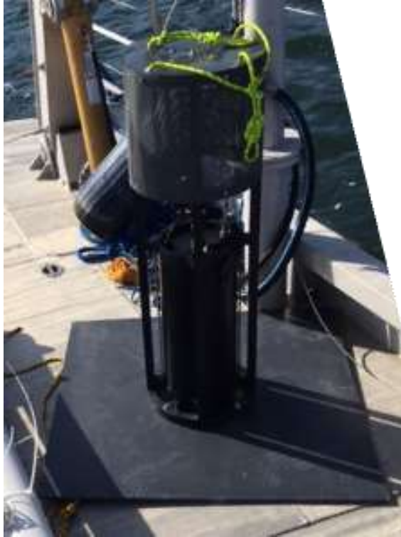
Figure 12: Instrument can, top to bottom: flow shield and sensor cage, instrument can, and drogue
