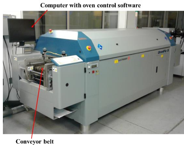
Figure 4.21 Reflow oven used for PCB/Copper plate soldering.
