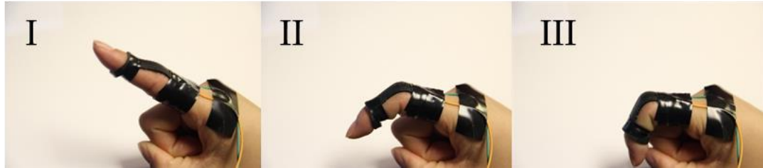
Figure 39. Images of a bending sensor on a finger-ring mounted on the forefinger, in straight (I) and bent (II and III) positions
