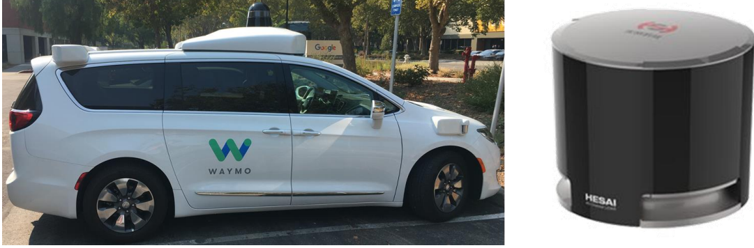
Figure 1. Waymo car with Lidar on top (left). Close-up of a Lidar sensor (right).
