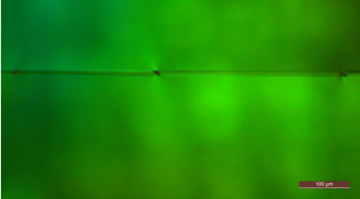
Figure 3.2: Polarized microscopy image of post-tested SFF sample with a single BF and three fracture events.
