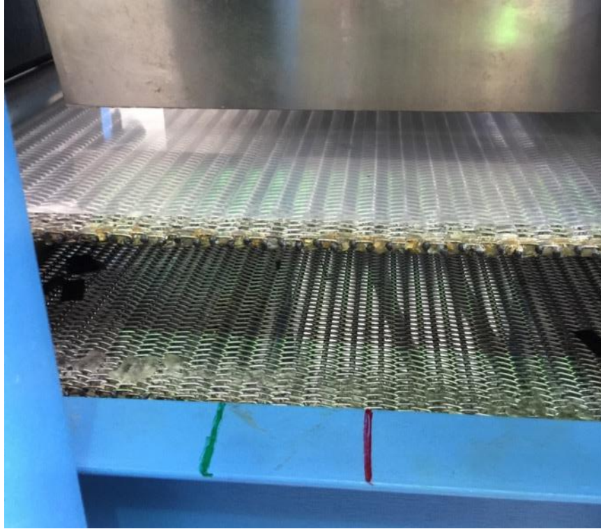
Figure A.7: Markers to start pouring the resin in the upper doctor box (green) and to start the cutter (red).
