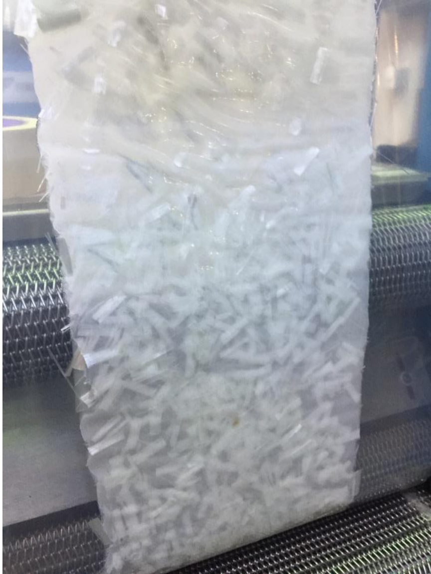
Figure B.4: Wet fibers stuck together in continuous SMC plate coming out of the SMC line.
