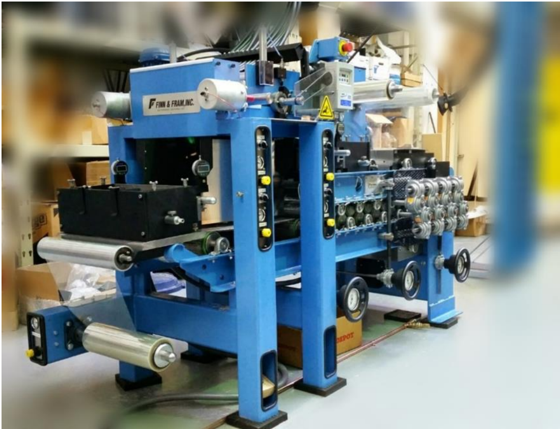
Figure 2.1: Sheet molding compound (SMC) production line used in this work.
