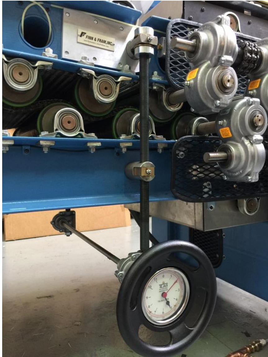
Figure A.6: One of three hand wheels for the adjustment of the compaction zone.
