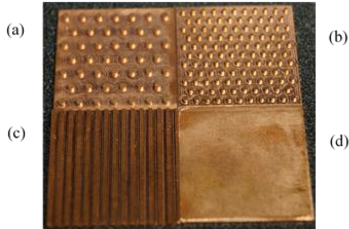
Figure 38 – DBC HS Designs, (a) Design 1 (MD MPF), (b) Design 2 (HD MPF), (c) Design 3 (Linear Channels), (d) Design 4 (Unstructured Channels)
