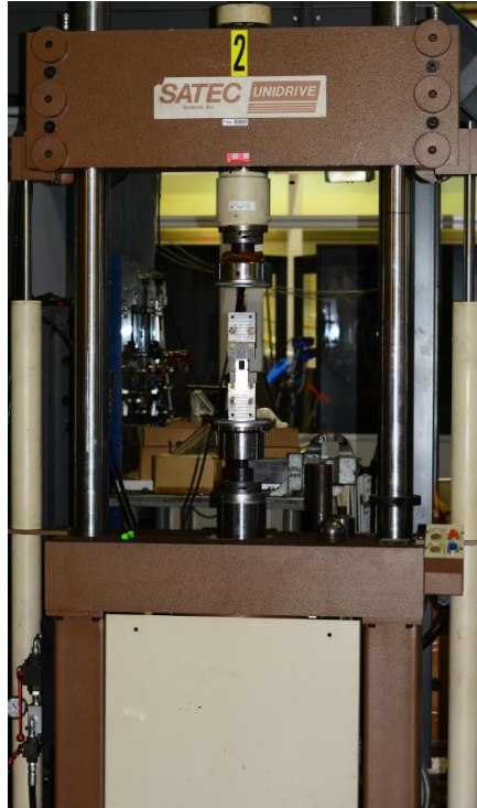
Figure 5.6 SATEC UNIDRIVE Hydraulic Testing frame
