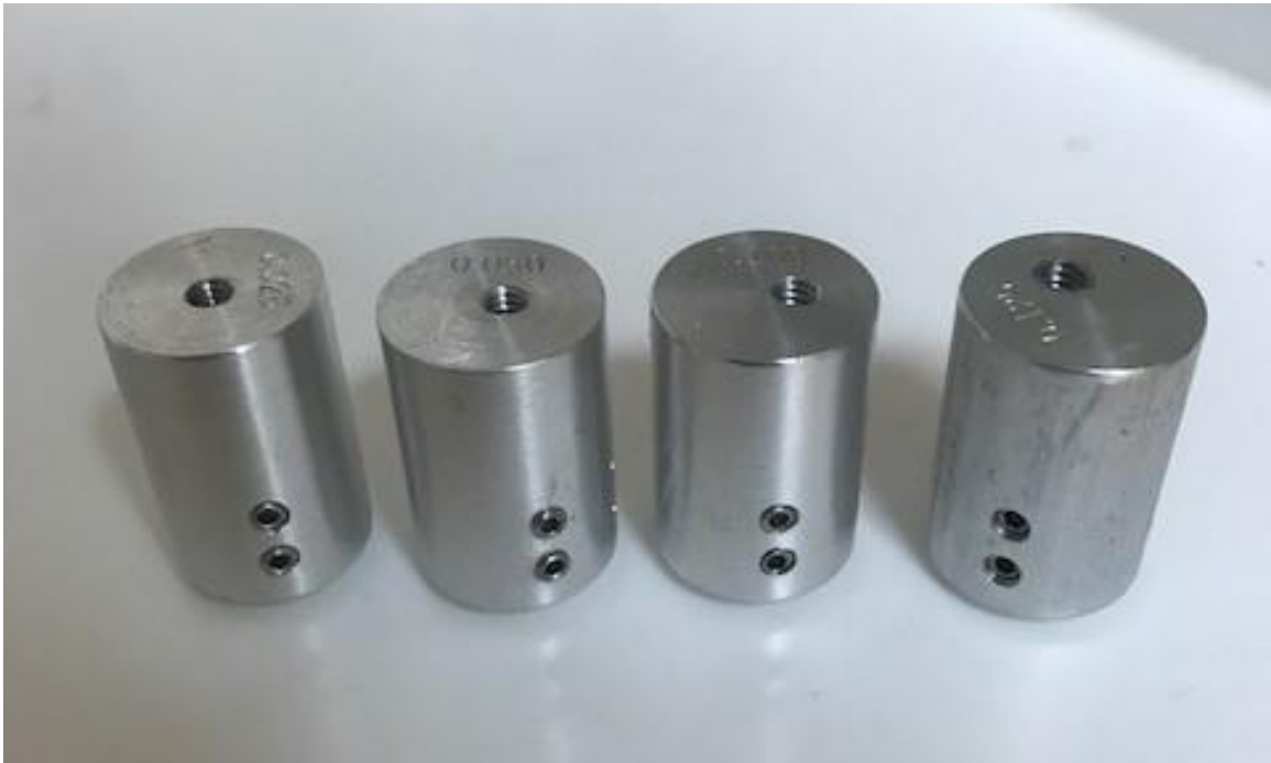
Figure 7 - Offset cranks that determined the levels of motion for the device
