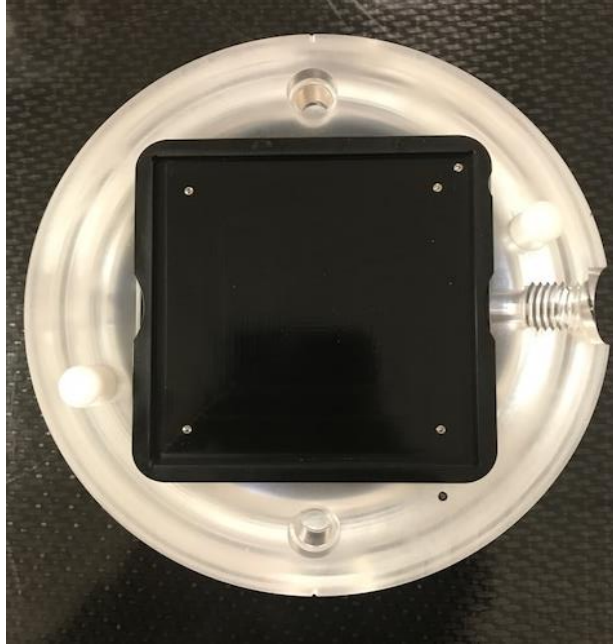
Figure 11 - Overhead view of the film cassette insert inside of the Lucy phantom
