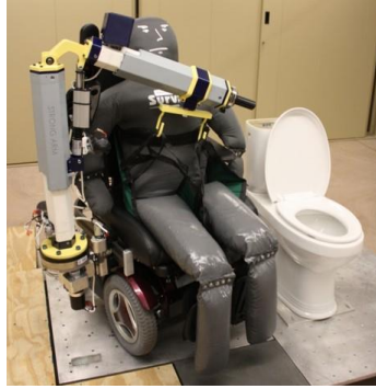
Figure 14: UPitt/QoLT Strong Arm power chair mounted patient transfer assist device [(30)]
