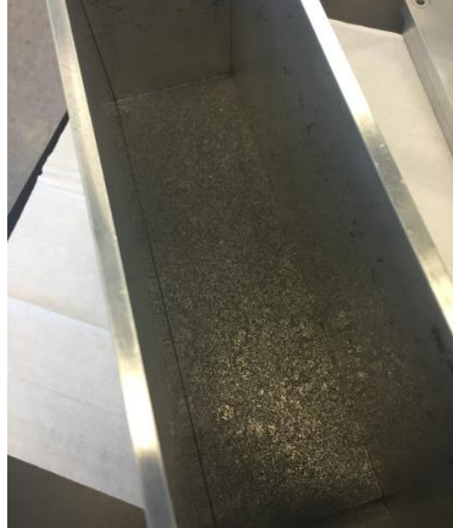
Figure 5.11. Schematic of mold and plunger (left); Compressed graphite in mold (right).
