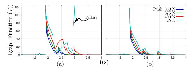
Figure 6.10: Push recovery comparison via the Lyapunov functions for IO (a) and ISS (b) based controllers.  $\varepsilon = \overline{\varepsilon} = 0.1$ . The convergence rate is preserved for ISS-CLF.
