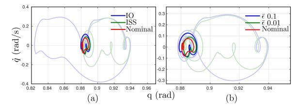
Figure 6.12: Walking over 5 cm step height. Phase portraits for vertical z position of the torso base are shown here. The ISS based controller shows a much smaller deviation.
