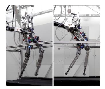
Figure 6.7: The spring-legged planar running biped, DURUS-2D.
