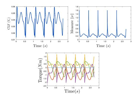
Figure 8.2: The RES-CLF (a), the measure (b) and the torque (c) as a function of time.  $\dot{V}_{\varepsilon}$  (slope of  $V_{\varepsilon}$ ) crosses 0 in every step, but the CLF is still seen to be ultimately bounded. It can also be observed that  $\|\nu\|$  increases when the torque inputs are high.
