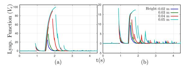
Figure 6.11: Step over comparison via Lyapunov functions for IO (a) and ISS (b) based controllers.  $\varepsilon = \overline{\varepsilon} = 0.1$ . The convergence rate is preserved for ISS-CLF.
