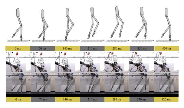
Figure 9.7: Running tiles of simulation vs experiment for the running robot DURUS-2D. Video link to the experiment is given in [6].
