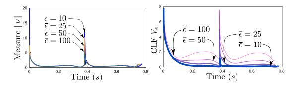
Figure 8.3: Progression of the measure, RES-CLF from the same initial point for different values of the auxiliary gain  $\bar{\varepsilon}$  is shown in the figure. It appears that the ultimate bound decreases with the auxiliary gain  $\bar{\varepsilon}$ , thereby nullifying the effect of uncertain dynamics.
