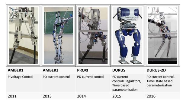
Figure 1.4: Progression of the walking controllers used on the robots over the years in AMBER Lab. From left to right: AMBER1, AMBER2, PROXI, DURUS humanoid, and the running robot DURUS-2D.
