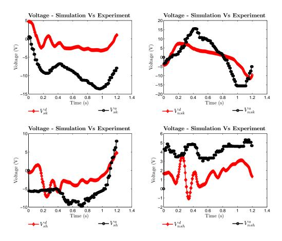
Figure 7.5: Figures showing the comparison between the voltage inputs obtained in simulation and experiment. The gap is less than 15V.
