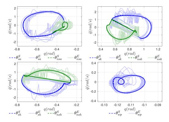
Figure 9.4: Phase portraits of the ankle, knee, hip and waist pitch angles of the robot. Both simulation (S) and experimental (E) results are shown.
