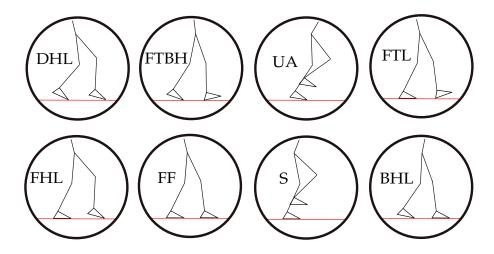
Figure 4.3: Representation of different possible domains for bipedal robotic dancing of AMBER2: double heel lift, front toe back heel lift, underactuated, front toe lift, front heel lift, flat footed, swing, back heel lift. There are eight possible vertices.
