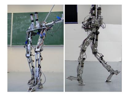
Figure 6.3: The bipedal robot AMBER2 (left) is constructed with the specific goal of multicontact behavior as indicated by the design of the feet (right).
