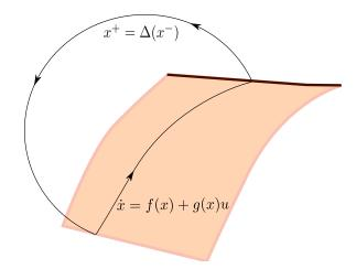
Figure 1.2: Pictorial representation of a hybrid system with a single continuous and a single discrete event. The continuous event is affine in controls, and the discrete event does not have a control input in this case. This type of hybrid system belongs to a class called *systems with impulses*. x is the state, u is the control input.
