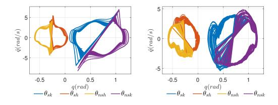
Figure 9.5: Limit cycles of simulations (left) and experiment (right), are shown for the running robot DURUS-2D. Both used the time based desired outputs:  $y_2^d(t) = y_2^d(\tau(t), \alpha)$ .
