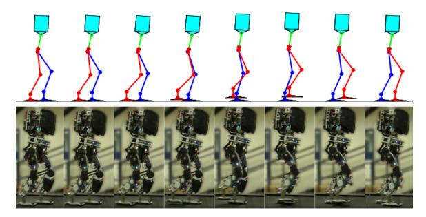
Figure 9.6: Figure showing the walking tiles of DURUS humanoid for one step. Video link to the experiment is given in [5].
