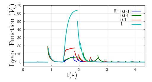
Figure 6.9: Comparisons of the Lyapunov function for various values of  $\bar{\varepsilon}$  for push recovery. The push force was 350N. The convergence is quicker for decreasing  $\bar{\varepsilon}$ . The jumps are due to discrete events (impacts).
