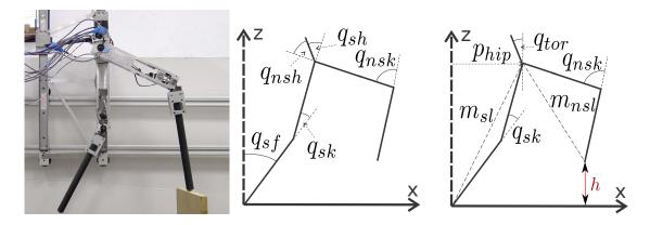
Figure 6.2: The biped AMBER1 (left) and the stick figure showing the configuration angles (middle) and output constraints (right).
