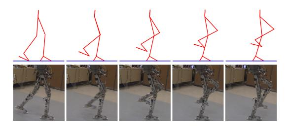
Figure 10.3: Tiles of a leg swing behavior consisting of a transition from back heel lift to swing pose. The top tiles illustrate the behavior of the robot achieved in simulation, and the bottom tiles show the same behavior realized experimentally on AMBER2.
