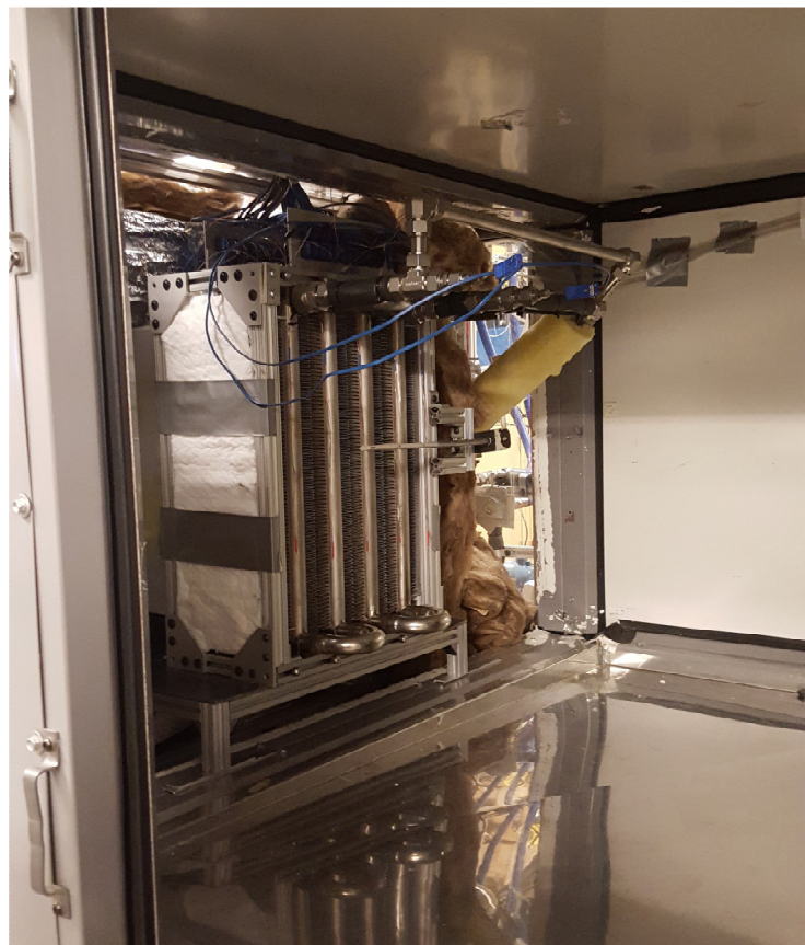
Figure 3.14 Test section mounted within wind tunnel test facility
