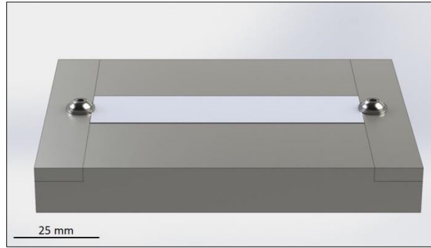
Figure 4-2 Almen strip fixture.
