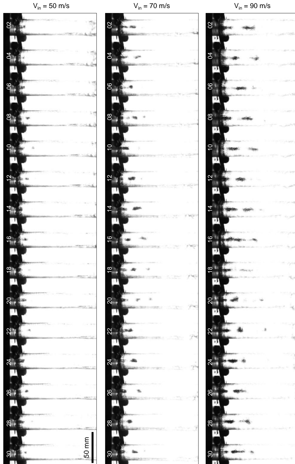
Figure 4-38 High speed video imaging of the cavitating flow for different inner jet velocities V_{in} . Video is captured at 14000 fps and frames are shown at 7000^{-1} \text{ s} ( 143 \mu\text{s} ) intervals ( V_{out} = 11.0 \text{ m/s} , frame numbers shown).
