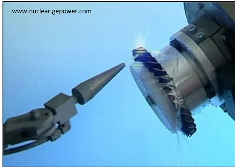
Figure 2-3 Water jet peening (WJP).
