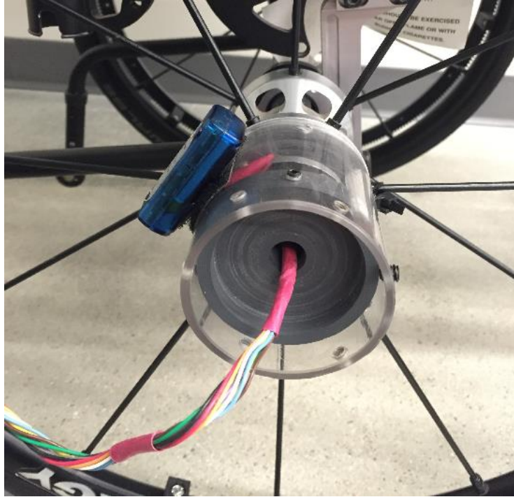
Figure 17. Accelerometer Mounted on Digital Encoder for Validation Testing
