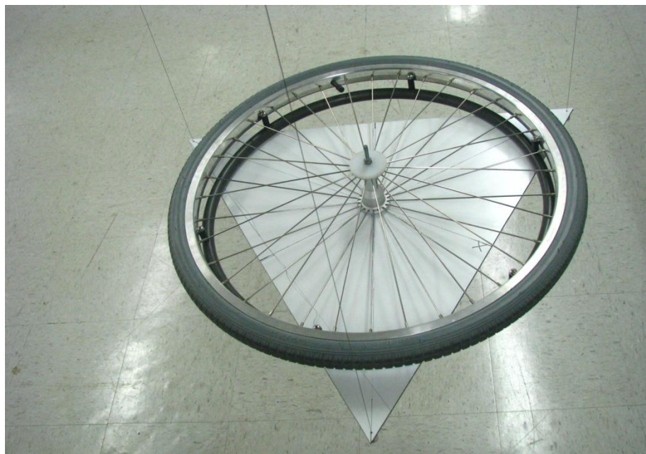
Figure 4. Drive Wheel Rotational Inertia Measurement by Trifilar Pendulum
