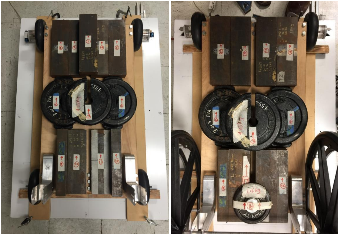
Figure 15. Cart 60%WD Configurations for Caster and Drive Wheels
