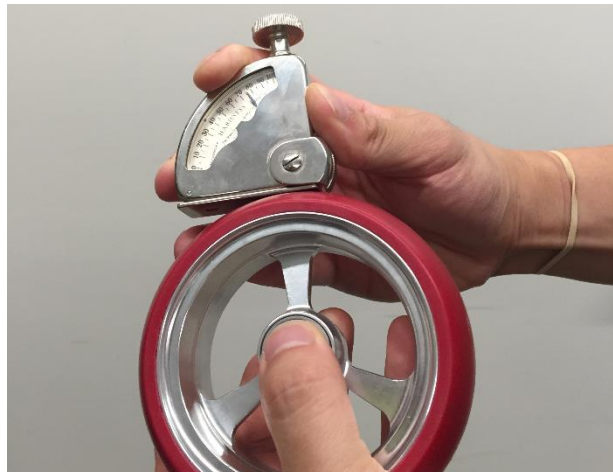
Figure 1. Durometer measurement of tire hardness
