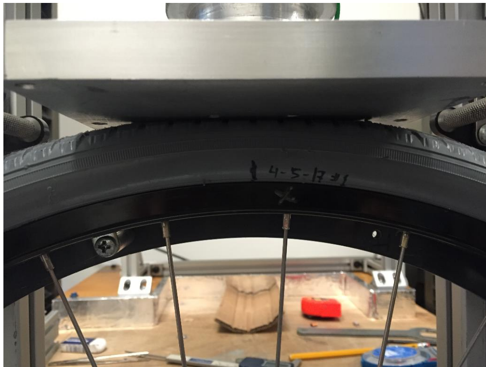
Figure 27. Drive Wheel Contact Patch on Surface Mounting Plate
