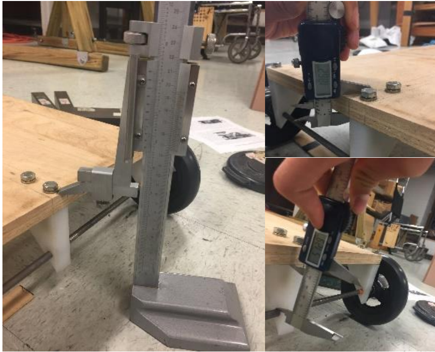
Figure 14. Measurement of "Control" Wheel Loaded Radius
