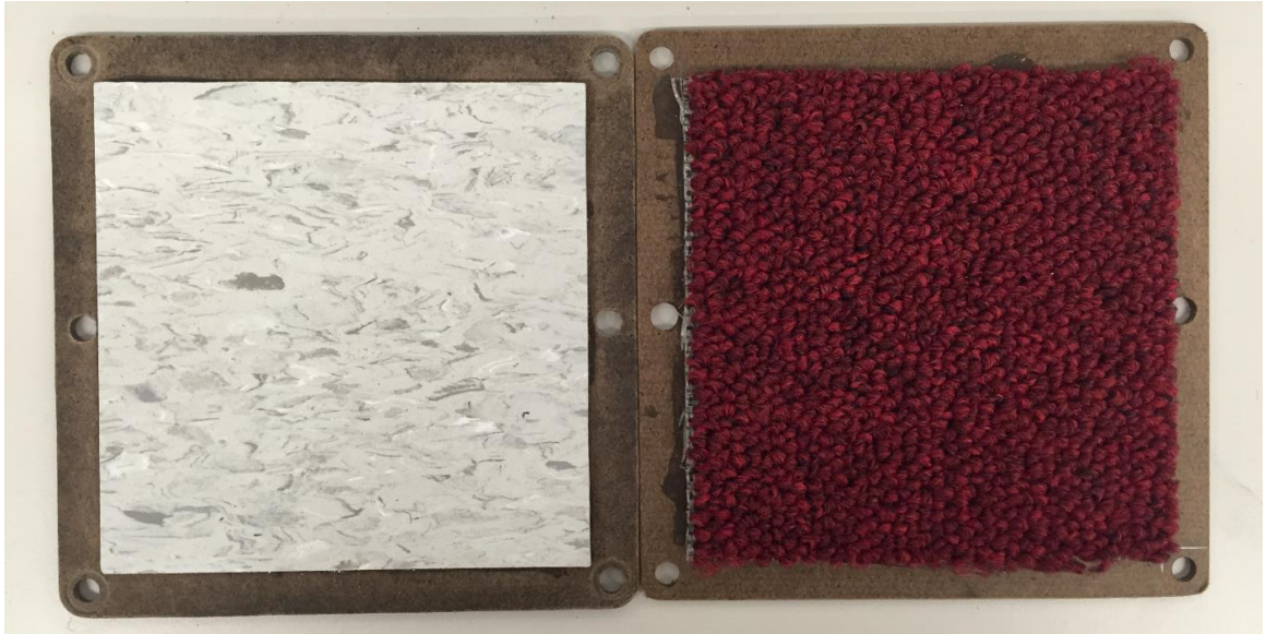
Figure 31. Tile and Carpet Scrub Torque Test Surfaces
