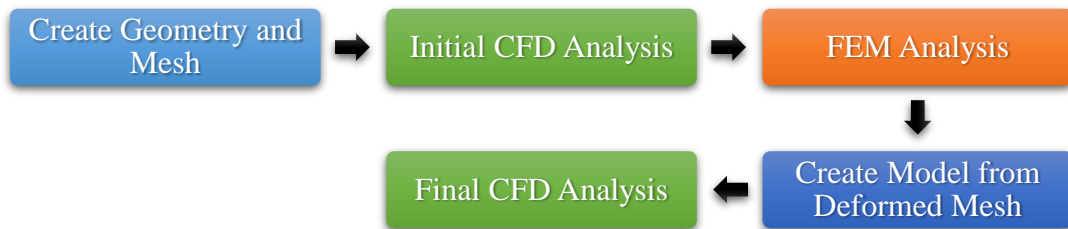
Figure 4.14. Workflow for the thermo-mechanical numerical model with one-way CFD/FEM coupling.
