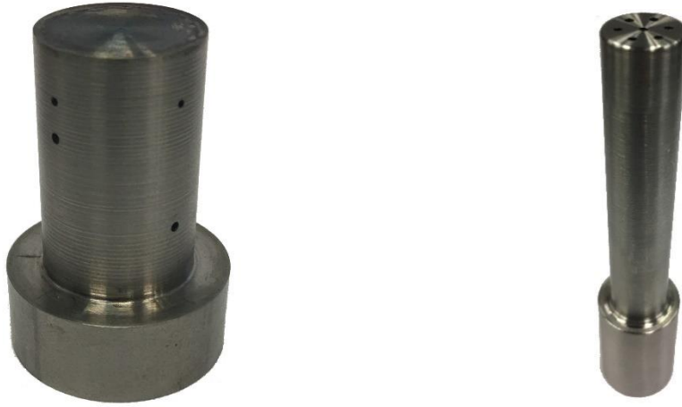
Figure 5.5. Pictures of the WL10 outer shell (left) and steel jets cartridge (right) for the optimized flat design.
