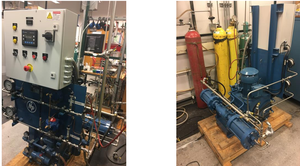
Figure 3.8. Pictures of the front (left) and back (right) of the reciprocating compressor.
