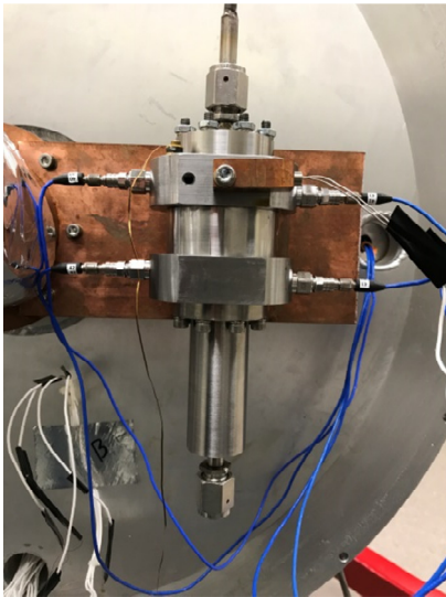
Figure 13. Experimental test section mounted to cold head with attached dynamic pressure transducers
