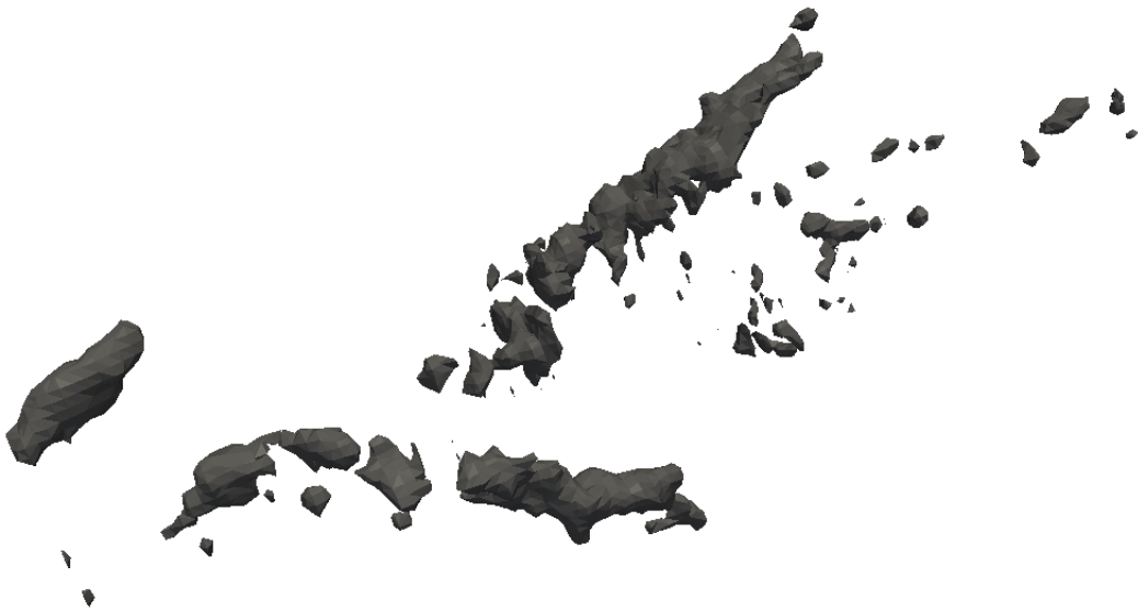
Figure 2.14 CAD rendering of inclusion imaged in figure 2.13. Note the presence of several small inclusions and the complex geometry. Use of a complex-geometry sample in the simulation demonstrates the filter performance on realistic, non-idealized data.
