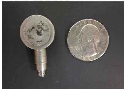
Figure H.1 Force transducer employed in impact experiments.
