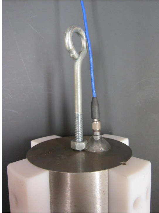
Figure H.4 Impactor with accelerometer attached.
