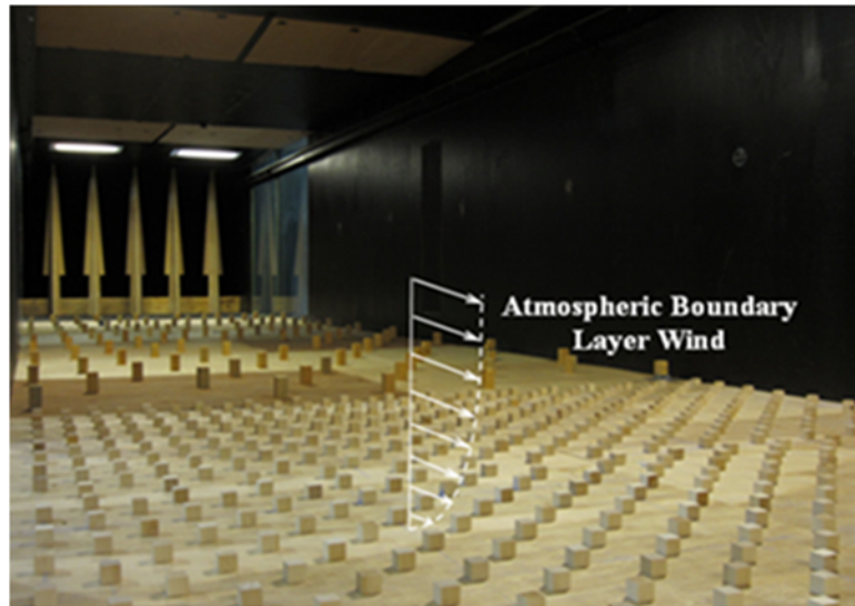
Figure 6-1 The test section of the AABL wind tunnel
