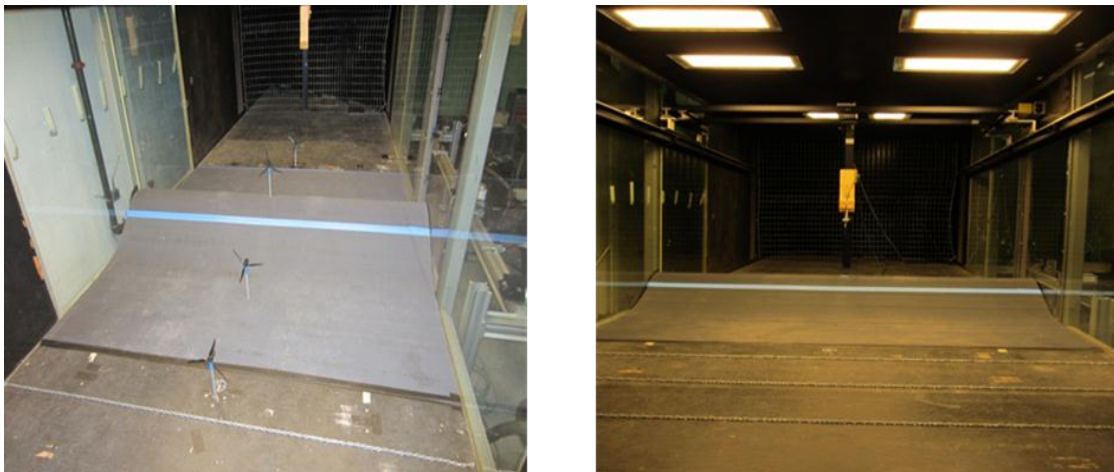
Figure 3-4 2D-Ridge profile with wind turbines installed around the ridge (left) and cobra probe measurement set-up on the top of the ridge (right)
