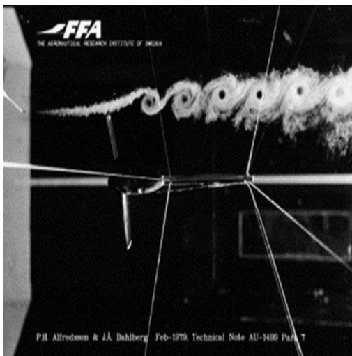
Tip vortices visualized with smoke (Alfredsson et al., 1979)
