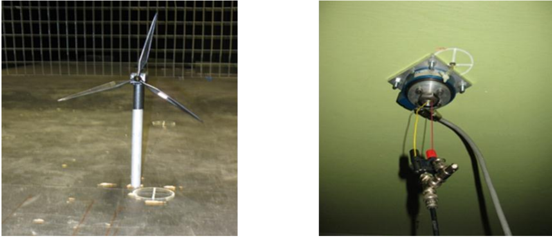
Figure 2-3 Wind turbine model (left) and force transducer and wiring equipment underneath of the model wind turbine (right)
