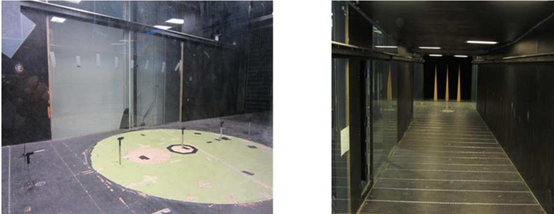
Figure 4-3 Five turbines in tandem arrangement with 3D spacing (left) and spires at the onset of the test section of the wind tunnel (right)
