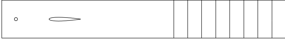
Figure 3.4: The permeable FW-H integration surface used for farfield noise prediction using the Charles simulation data. The “endcaps” remove numerical errors (expected to be uncorrelated over the end surfaces) through the integration process.
