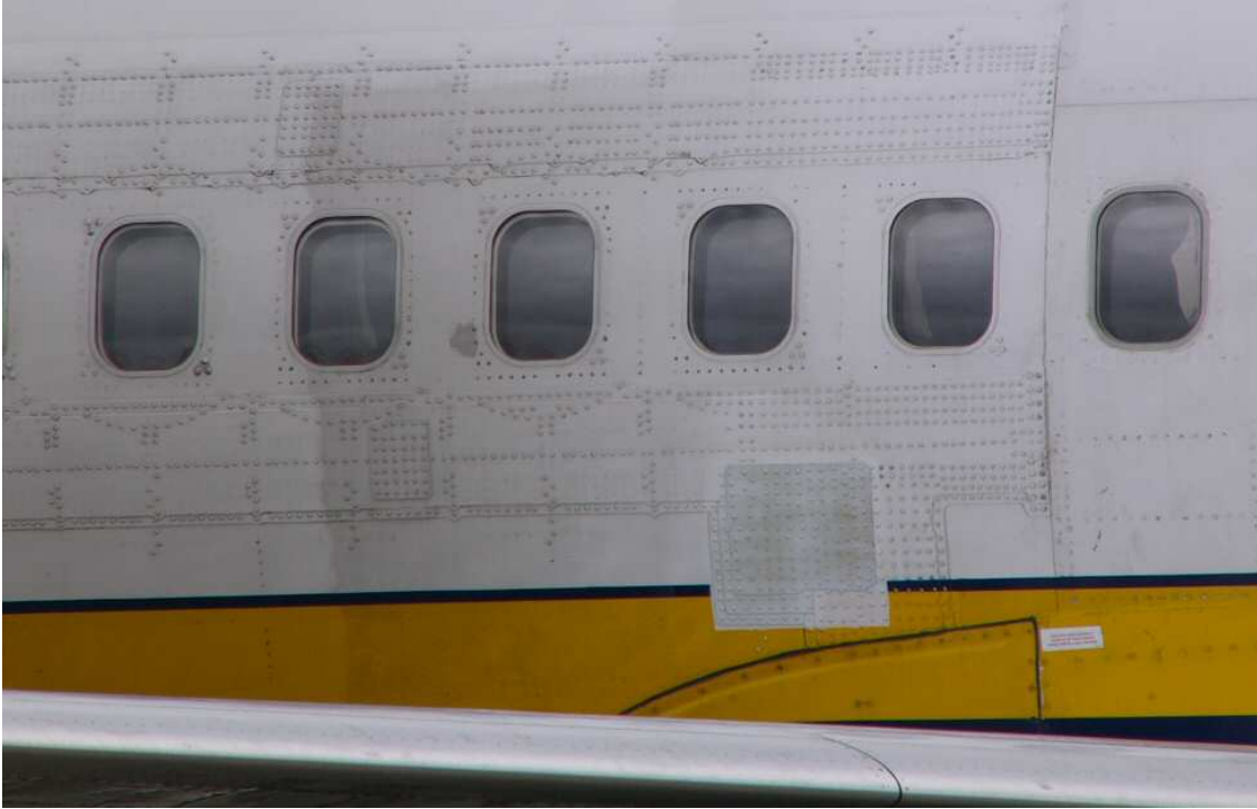
Figure 1.3: Riveted lap joints on the fuselage of Boeing B737 (Courtesy: Boeing Company)
