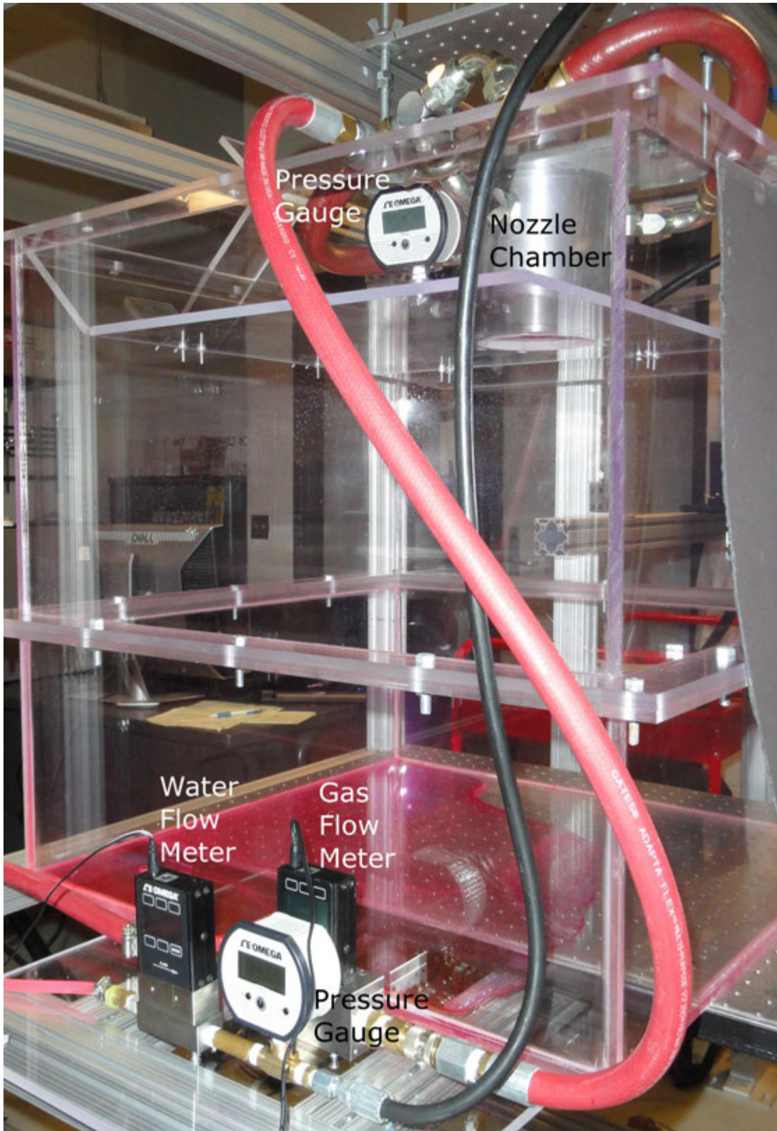
Figure 3.2 Experimental Test Setup, Flow Meters and Pressure Gauges
