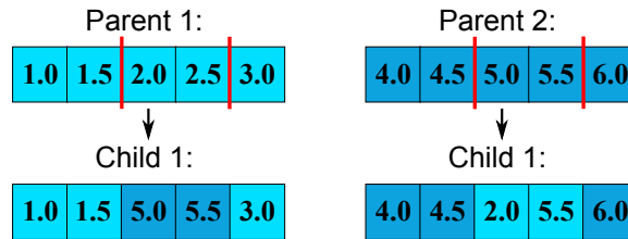
Figure 4.3 Illustration of the double point crossover with the 3rd and 5th variables chosen as the crossover point.
